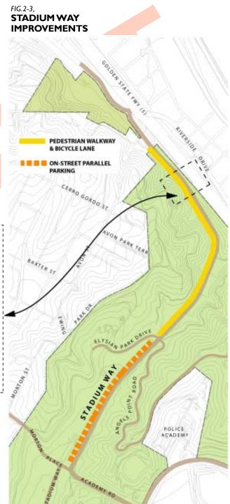
THE PROPOSED LANE CLOSURE ON STADIUM WAY, FROM THE 5 FREEWAY EXIT TO ELYSIAN PARK DRIVE, WOULD ALLOW THE CONSTRUCTION OF A PEDESTRIAN WALKWAY AND A CLASS 2 BICYCLE LANE. SEE FIG. 2-2, LANE RECONFIGURATION DIAGRAM.
